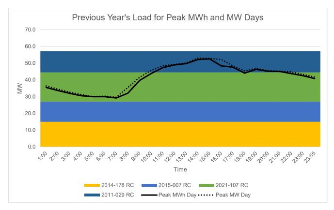
Peak MW occurred on 14:00 due to all commercial and industrial loads were operating at its peak during this time. Peak daily MWh occurred on 14:00 for the same reason. As shown in the Load Curve, the available supply is higher than the Peak Demand.
