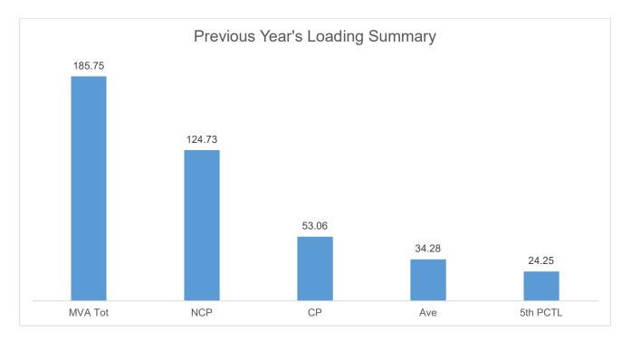
The Non-coincident Peak Demand is 124.73 MW, which is around 67.15% of the total substation capacity of 185.75 MVA at a power factor of 1.0. The load factor or the ratio between the Average Load of 34.28 MW and the Non-coincident Peak Demand is 27.48%. A safe estimate of the true minimum load is the fifth percentile load of 24.25 MW which is 19.44% of the Non-coincident Peak Demand.
