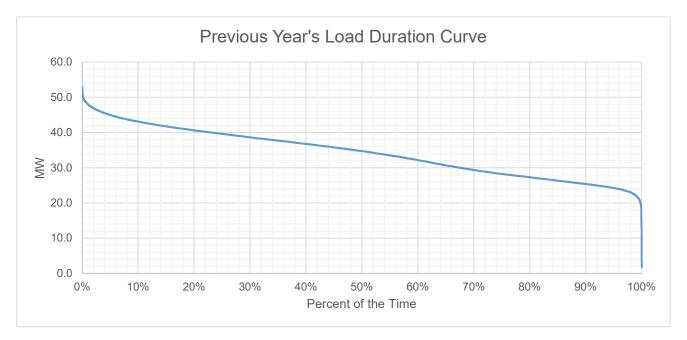
Based on the Load Duration Curve, the minimum load is 20 MW and the maximum load is 53.06 MW for the last historical year.
